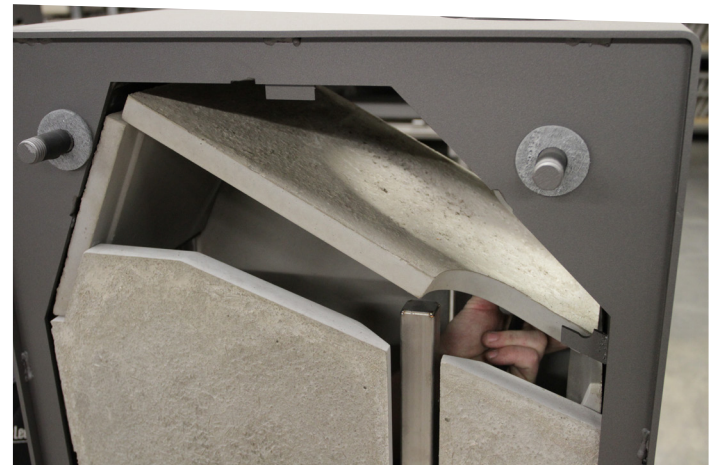
...or remove the bar on which the top reflection shield rests and let the soot residue slide of.
