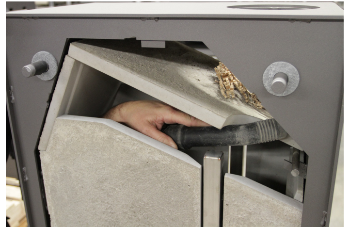
Use a vacuum cleaner to remove soot residue from the top reflection shield...
